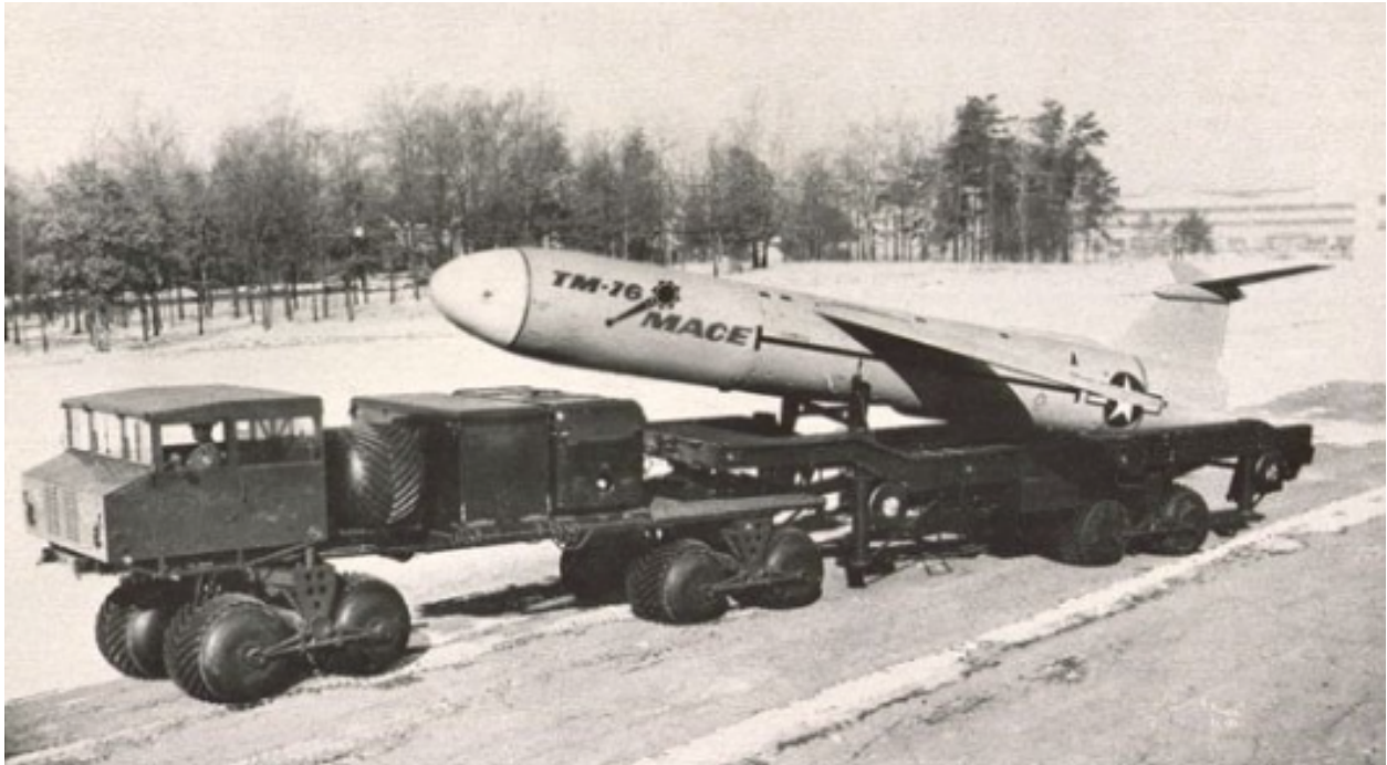
Ready and rearin' to go. The TM-76 Mace guided missile perched atop an MM-1 Terracruiser vehicle that can transport through desert, sand, swamp and snow to front line combat positions
